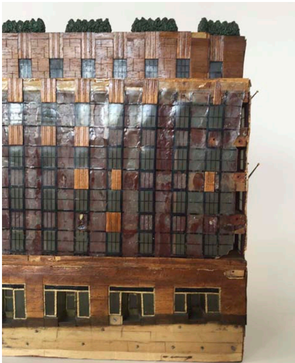
Fig. 18. England, with flattened and attached cellulose acetate. Visible at right of image is a void where the cellulose acetate sheet shrank due to loss of original plasticizers.
