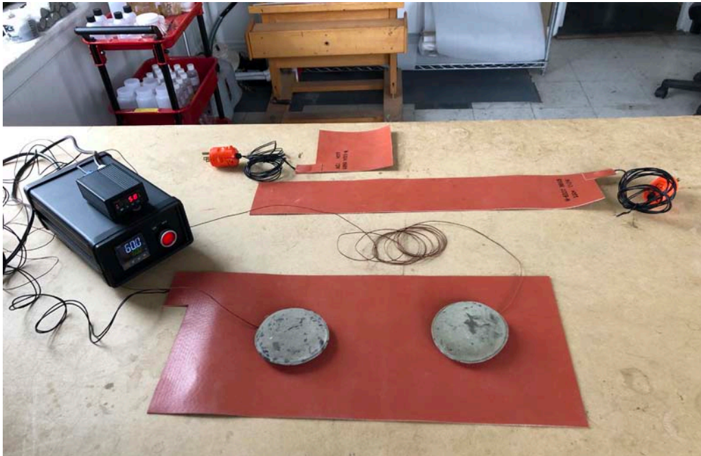
Fig. 8. Custom made silicone rubber heating mats, control box and external thermal couples manufactured by Instrumentors Supply.
