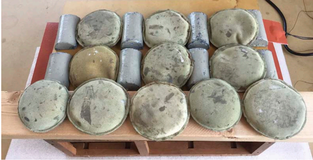
Fig. 17. England showing heating mats and weights used for flattening warped cellulose acetate.
