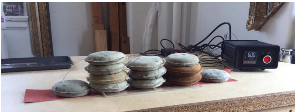
Fig. 9. Rainbow room, flattening warped cellulose acetate fragments using heating mat and weights.
