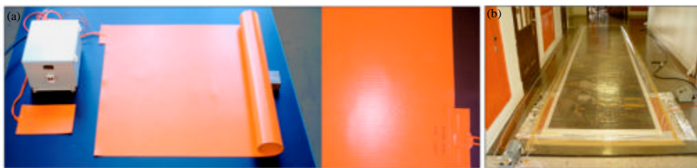
Fig. 3 (a, b): (a) Experimental Olsson-Markevicius silicone rubber and wound wire mild heater (2010) and (b) lining one of the H.S Sewell murals using vacuum envelope and flexible thermal blanket
